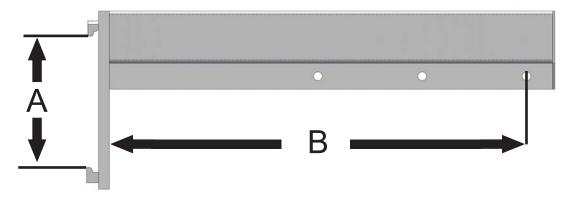
A - ITA Class II, III, IV, V or Pin mounting B - 24" up to 240" Capacities up to 50,000#
