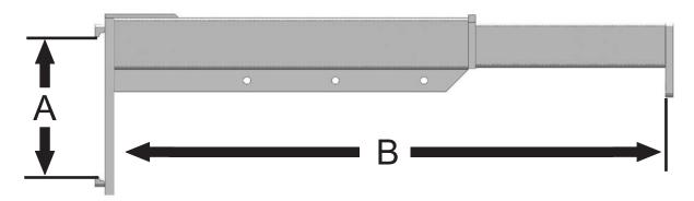
A - ITA Class II, III, IV, V or Pin mounting B - 48" up to 360" Capacities up to 50,000#
