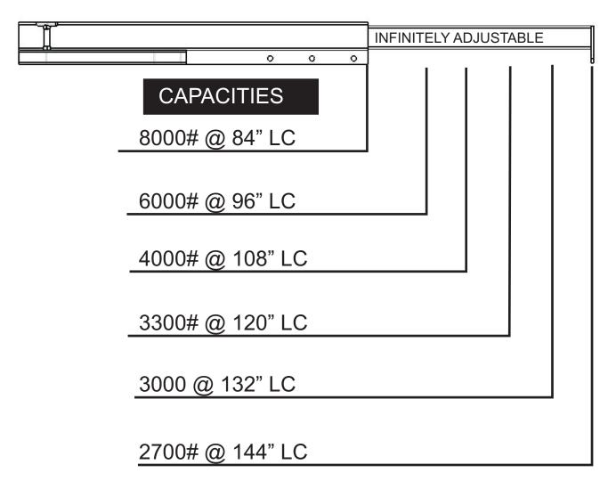
\*VERTICAL CG IS TAKEN FROM THE LOAD BEARING FACE OF THE FORK (TOP OF FORK)
