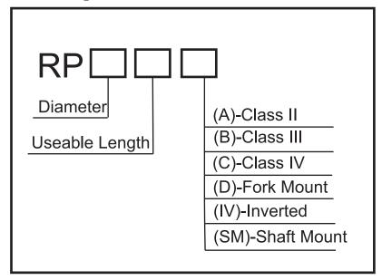
If the requested ram pole, is to be 2.75" diameter with a useable length of 120", Class II ITA Mount, then the model number would be RP2.75120A
